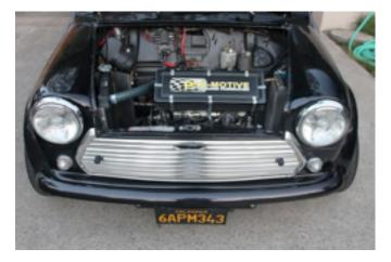
The builder started with a clean 1970 Mini. The R1 Yamaha engine is a 2003 5PM fuel injected mill rated for 170hp, with a redline of 12,500 RPM. A ground-up mod took place, with the suspension completely replaced with all aluminum adjustable equipment at the corners. The car now has dual radiators, the gearbox upgraded, and a Quaife LSD installed for good measure.
