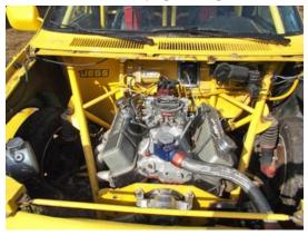
The vehicle no longer has the transverse mounted engine, nor the front wheel drive setup. Within the custom hood and front end, the SBC is a stroked out 355 CHEVY MOTOR TURBO 400!!! mated to a TRANS 3500 CONVERTER!! with a 9 INCH FORD REAR END!!! and 456 GEARS!!!
