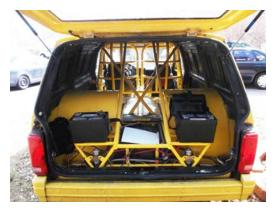
This monstrosity only has seating for 2 willing-or kidnapped-people. The cargo area is greatly reduced by the scratch-built round section tube frame and huge tubs for the rear wheels, with the batteries bolted behind for weight distribution.
